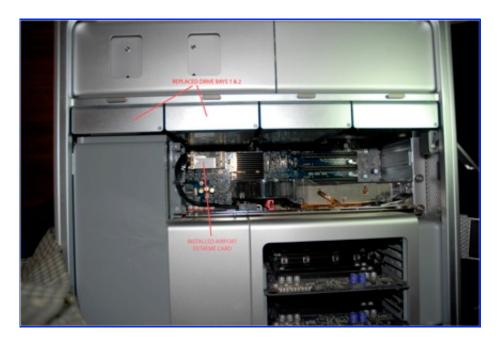
**8**. Reconnect the Mac Pro to the keyboard, mouse, monitor and network and boot. On the Apple Menu check "About this Mac" to confirm that the Airport Extreme card is being recognized.
