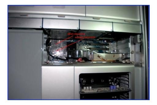
**3**. Remove hard drive bays 1 & 2 to give yourself some extra room. The latch in the back that was used to remove the side panel will have to remained released to remove the drives bays. The drive bays pull straight out once this latch is released.
